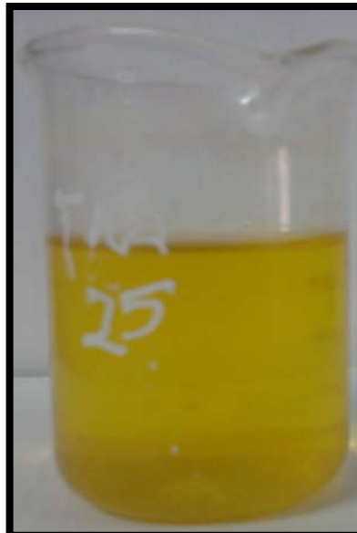
Methyl Jojoboate (biodiesel) and Traces of glycerin after settling
