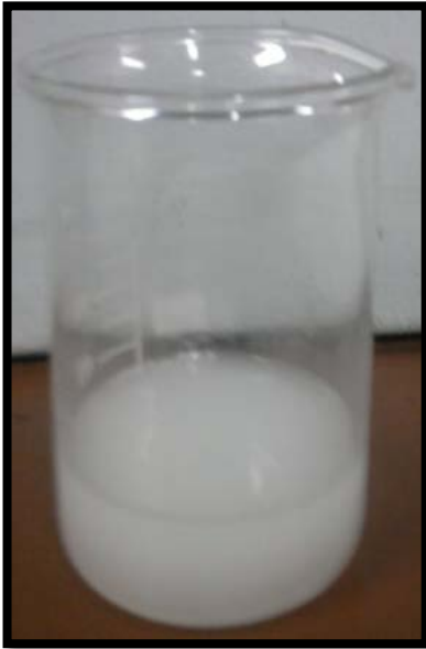
Methanol with potassium oxide forming methoxide
