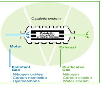
the conventional manner and finally to atmosphere. The catalytic converter's purpose is to reduce the original harmful emissions to negligible levels by means of catalyst controlled chemical reactions. Within the structure of the catalytic Converter is a form utilizing a catalyst.
