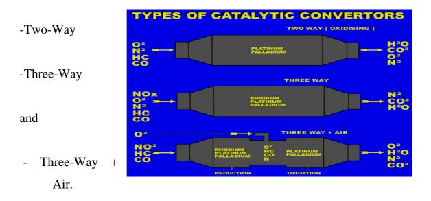
Each type uses a slightly different method and chemistry to reduce the harmful elements in exhaust emissions. Early model converters used a palletized catalyst, but most modern converters are now designed with a freeflowing honeycomb ceramic catalyst. The type of converter required on a particular vehicle varies with model year, engine size and vehicle weight. Some vehicles even make use of more than one type of converter or a preconverter to meet emission reduction standards.
