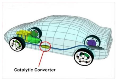
converter where an almost total degradation of exhaust smoke can be achieved by catalytic reactions over a hyperactive area made of platinum and rhodium. In spite of its modest volume, the active surface area inside a catalytic converter would cover two football fields  $(^3)$ .
