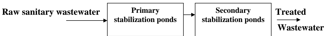
Figure (2- b) processing diagrams of system for treatment of small wastewater flow - Natural biological stabilization in ponds.
